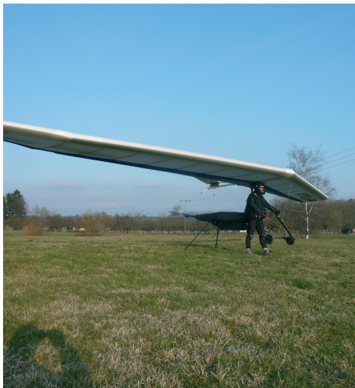
A new era for powered hang gliding: this Atos is powered by an electric motor from Toni Roth, which gives him 15 minutes to fly up to the thermals.
